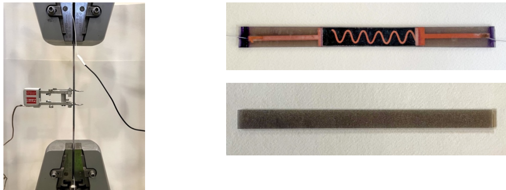
Figure 7: Left: Uniaxial tension test. Right: samples with sensor (top) and without (bottom).
