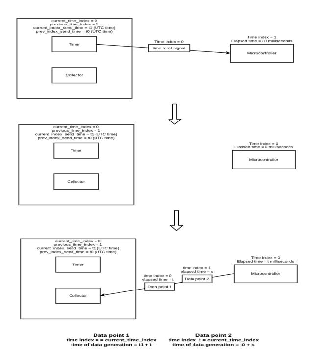
**Figure 6:** Sequencing Events/Keeping Track of Time – a reset signal, sent from the timer object with time index 0, changes the time index on the microcontroller to 0. The microcontroller transmits two data points – one of which was generated after the most recent reset signal (hence, the time index is 0), and the other one was generated before the most recent reset signal that is after the prior reset signal (hence, the time index is 1).
