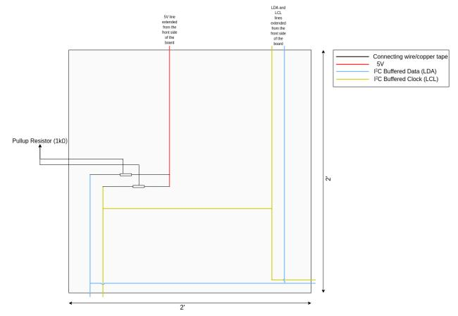
Figure 3.b: Circuitry on the back side of the prototype mural (svg file is available at this <u>link</u>)
