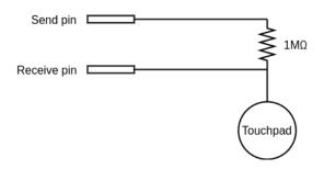
Figure 2: Circuit diagram for capacitive touch sensor
