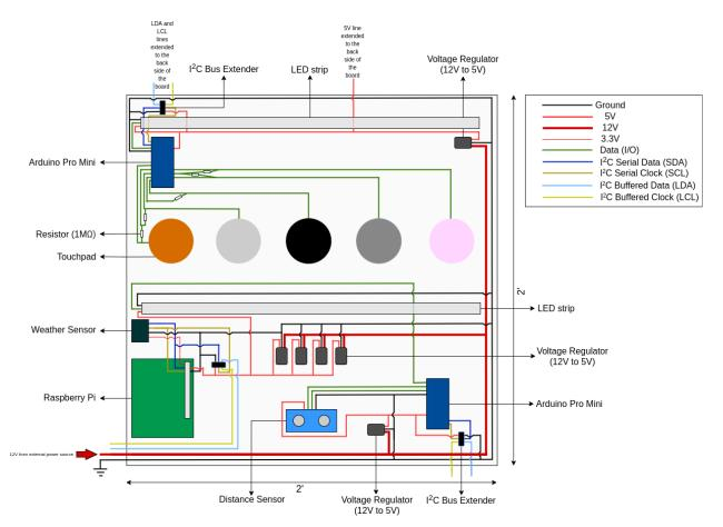
Figure 3.a: Circuitry on the front side of the prototype mural (svg file is available at this link)
