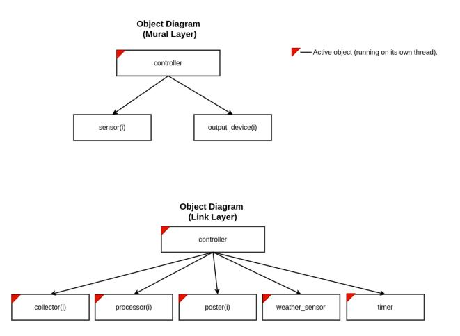
**Figure 4:** Object diagrams for the Mural Layer (top) and the Link Layer (bottom)
