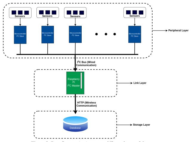
Figure 8: Data Communication across different layers of the system
