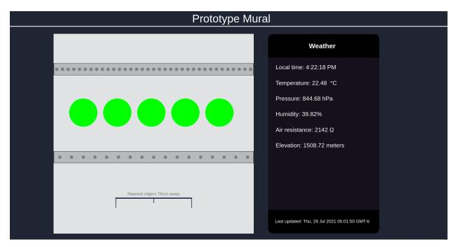
**Figure 5:** Web UI – a screenshot of the web page that renders real-time visualization of the physical interactions on the prototype mural remotely.
