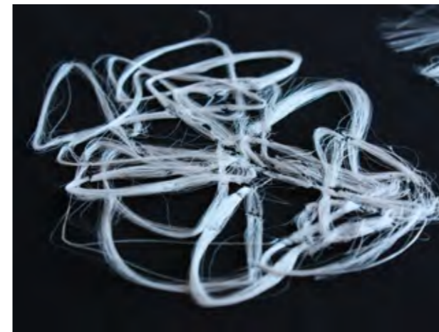
FIGURE 82. 'WELDED' PP YARN
