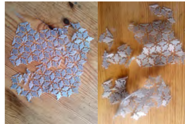
FIGURE 53. PLA SAMPLE BEFORE (L) AND AFTER (R) WASHING MACHINE
