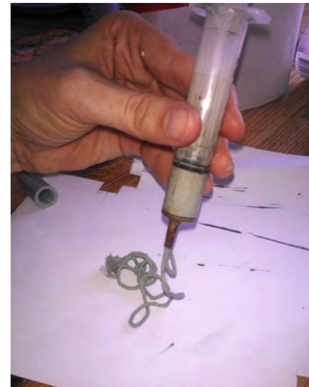
FIGURE 84. EXTRUDING THE CELLULOSE MIXTURE
