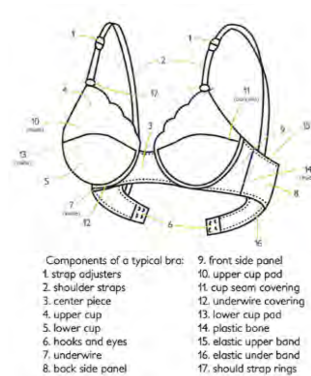
FIGURE 48. COMPONENTS OF A TYPICAL BRA [BASED ON CHAN ET AL. , 2001]
