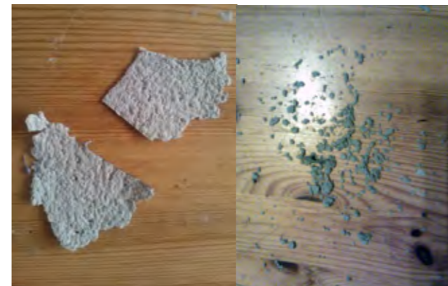
FIGURE 54. CELLULOSE SAMPLE BEFORE (L) AND AFTER (R) WASHING MACHINE
